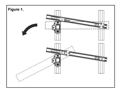
Metal Cabinet Installations: Install roller wheel assembly using the M8 hardware provided. (Figure 2) If using strut channel, use M8 strut nuts to ease adjustment (strut hardware not provided).
