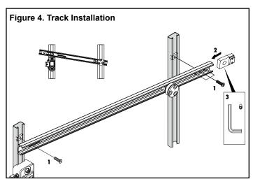
4. Reinstall track roller, rear bumper and end stop.
