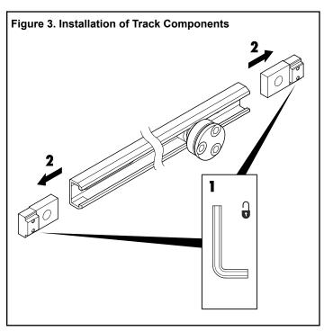
Install the track using M8 or 5/16" flat head bolts or machine screws (not included) at the front and rear of the track. Be sure the fasteners are flush with the track and do not interfere with track roller movement.
