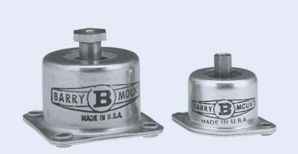
Barry B-Mounts provide shock and vibration isolation for avionic equipment in high performance aircraft. They feature low resonant transmissibility and isolate high frequency vibration without snubbing during high "g" maneuvers.
