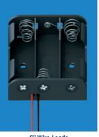
**6" Wire Leads**Allows battery holder to be place remotely from PC freeing up valuable board space.
