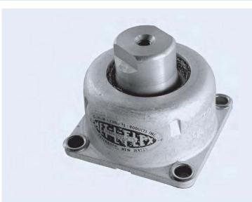
The high damping and nonlinear characteristics of MET-L-FLEX load carrying element and limiter pads in the all metal 1201 and 1202 Series Isolators assure controlled shock and vibration isolation protection for mounted equipment.
