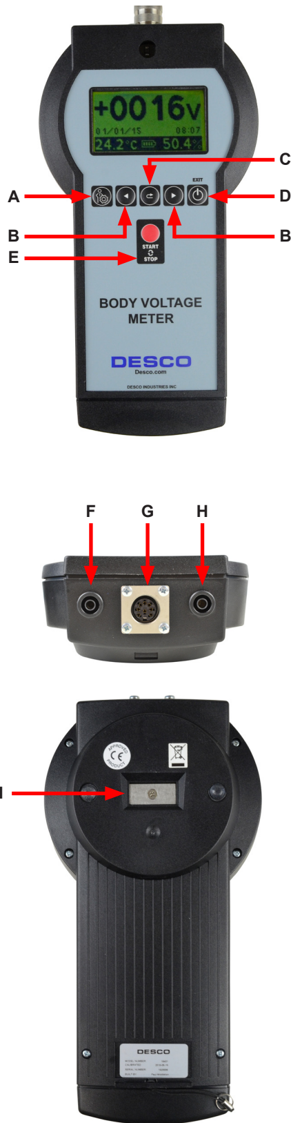
Figure 2. Body Voltage Meter features and components
